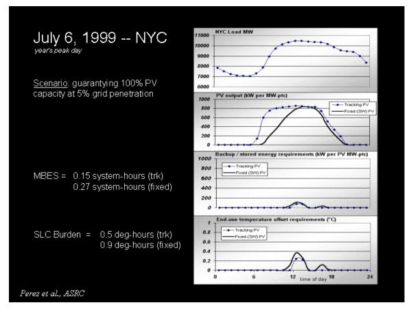
This diagram is an illustration of the most extreme load day in NYC on July 6, 1999. The grid was particularly stressed with heat and high energy transfers on that day, leading to the collapse of localized distribution systems. The top diagram represents the City's load shape on that day. The second diagram shows that the amount of solar resource was almost ideal on that day.
