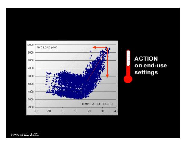
End-use temperature-based load control would be particularly effective in a place like New York City. The diagram above illustrates one year's worth NYC hourly electrical loads as a function of ambient temperature. The right side of the diagram shows that the City's load grows as a function of cooling requirements. Hence, any action on these requirements via thermostat adjustment would have an impact on the load.
