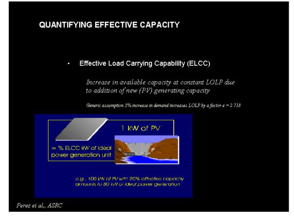
In order to measure the contribution PVs could make to a grid's available capacity, we used several complementary "yardsticks" to quantify effective capacity. The first of these measures is the Effective Load Carrying Capability (ELCC).
