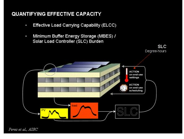
This slide illustrates how end-use load control could be implemented in response to local or regional PV output and load requirements.
