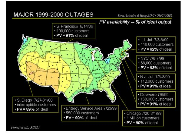
This diagram shows that, during all instances of heat wave-driven grid stress situations in the country, the availability of the solar resource was nearly ideal. The most recent data from 2001 fully confirm this observation (as of 6/20/01).
