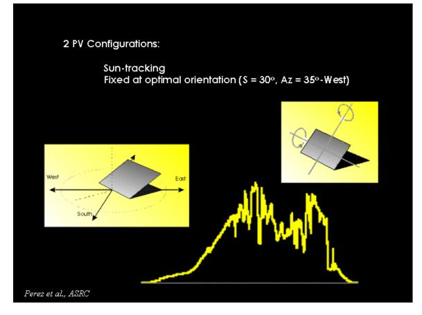
We considered two solar deployment technologies: (1) the ideal case: using sun-tracking solar arrays; (2) the practical case: using fixed solar arrays (i.e., the kind easily deployable on building roofs and other structures).
