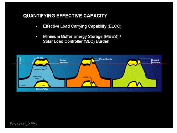
However, because the ELCC is a statistical measure that some may question, we define another yardstick that can be expressed either in terms of energy backup in the case of the minimum Buffer Energy Storage (MBES), or end-use load control in the case of the Solar Load Controller (SLC) Burden.
