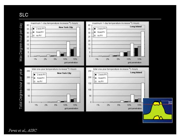
As above, the two left diagrams correspond to NYC and the right ones to L.I. The X-axis, again, represents PV penetration on the considered grids.
