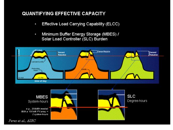
Sometimes conditions are not as ideal, so we looked at how much backup energy would be needed (middle diagram), or alternatively, how much end-use load control, i.e., consumption reduction, would be needed (right diagram), to guarantee that all resources above the red line are met.
