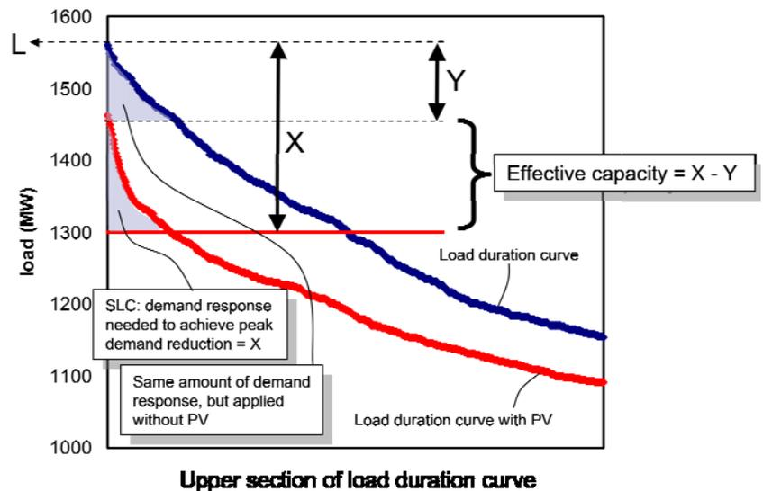
Figure 1: Illustrating the SLC effective capacity metric [11]
