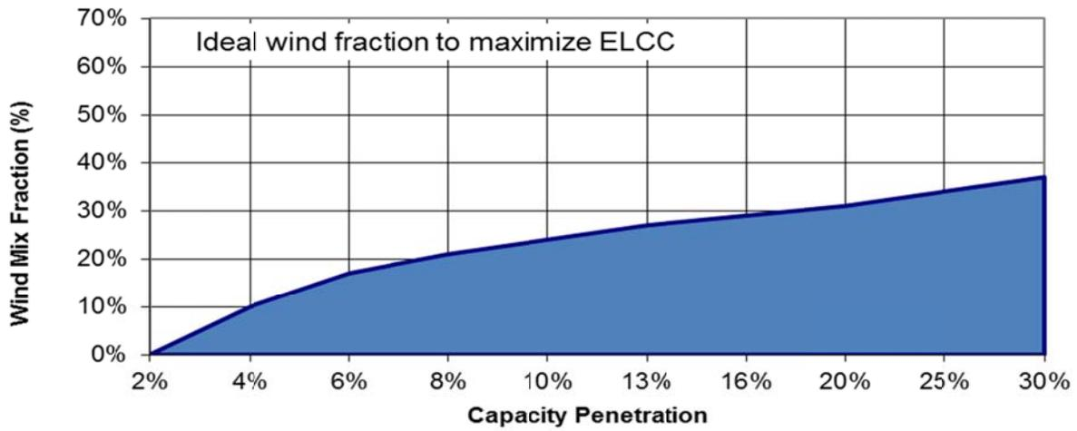
Figure 3: Ideal Wind fraction for the ELCC metric
